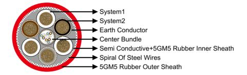
**System1 (1.8/3kV or 3.6/6kV):** Flexible stranded tinned copper conductor with heat resistant 3GI3 rubber based on EPR, easy strippable outer conductive layer.
